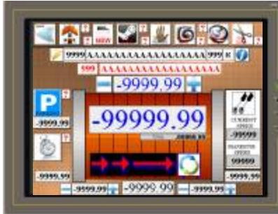
**Colour touch screen**—a 12" touch screen (left) makes for simple setup, and the powerful computer provides the user with a choice of up to 5 different operating languages. The logically arranged programming screens clearly display every function that the operator might need.
