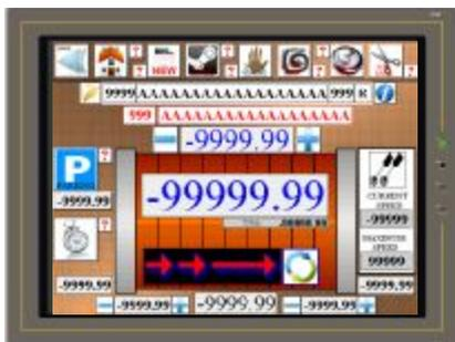
**Colour touch screen**—a 12” touch screen (left) makes for simple setup, and the powerful computer provides the user with a choice of up to 5 different operating languages. The logically arranged programming screens clearly display every function that the operator might need.
