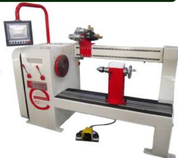
**4-ratio quick change spindle drive**—provides maximum versatility for fast primary winding at high speed, whilst smoothly delivering the necessary torque at lower speeds.
