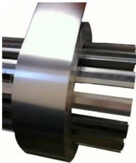
**Expanding mandrels** (left) are available for all types of foil and strip, including copper and aluminum. Custom built to our own designs, these are optimised for speed and ease of operation in the workplace.
