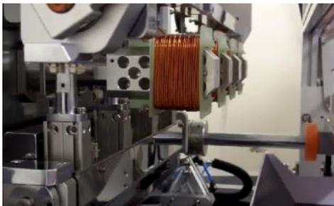
A recent delivery from IWM, producing EI-84 transformers on a 4 spindle machine with automated loading and unloading of bobbins.
