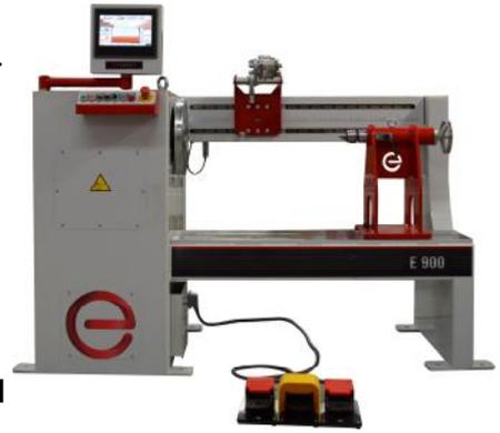
**Two-speed gearbox with electronic gear change** — provides maximum versatility for fast winding at high speed, whilst smoothly delivering the necessary torque at lower speeds.
