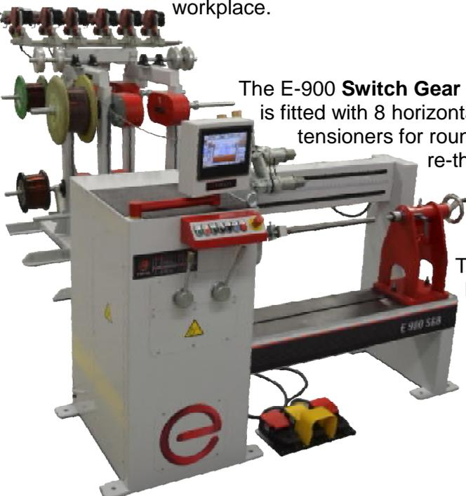
The E-900 **Switch Gear Box** machine (left), is set up for maximum **versatility**, this example is fitted with 8 horizontal despoilers for profile wire and 6 programmable electronic tensioners for round wire. A wide range of transformers can be made without having to re-thread the wire - simply change the tooling and switch program, and you're ready to wind.
