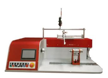
There are various configurations of speed ranges, up to 9,000 rpm (depending machine version). This produces a fast cycle time for high turn primary windings.
