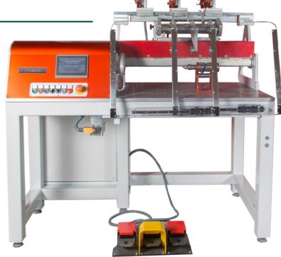
There are various configurations of speed ranges, (depending machine version). This produces a fast cycle time for high turn primary windings.
