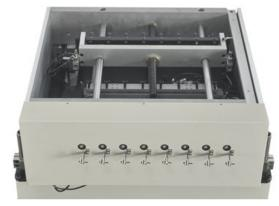
When making a solder connection to fine wire, the mechanical strength of a single strand of wire may not be sufficient. The skeining unit reinforces the start and finish leads of the winding by twisting multiple strands of the wire together, so that they can withstand the soldering process.
