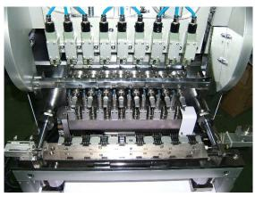
For cutting larger wire diameters the pin tear method will no longer work. In this case we can fit air operated cutters close to the nozzle head.
