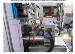
Allows automated load and unload, improving the machine throughput/cycle, and allowing easy access for extra stations to be added to the line, e.g soldering, welding etc.
