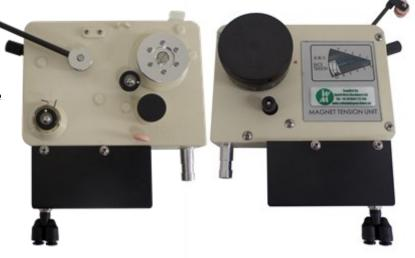
The models shown have a pneumatic cylinder (controllable from the winding machine) for tension release as required during pin wrapping operations as well as microswitch detecting arm moving up indicating wire brake.
