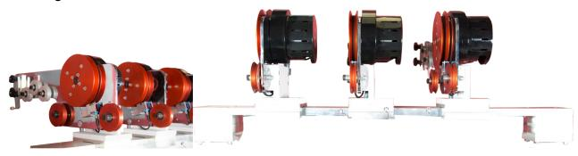
The tension is controlled from the machine's operating software, setting the desired tension independently for each winding and stored with that program / coil setup.
